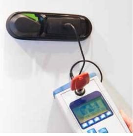
Programming unit – transfers authorizations, reads logs or opens doors if batteries run out.
